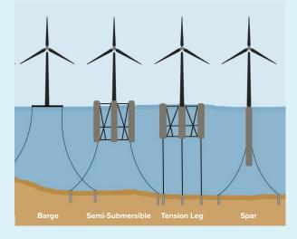
Tension Leg and Spar. The foundation type will be decided on during the wind farm design phase.
